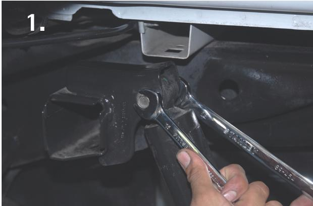
1. With the vehicle safely supported with jack stands start by removing the upper shock mount bolt using a 15mm wrench on the bolt and a 18mm socket or wrench on the nut.
