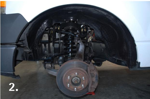
With the vehicle level on the ground set the emergency brake and block the rear tires. Using a floor jack, raise the front end and support the frame rails with jack stands for safety. Then remove the front tires.
