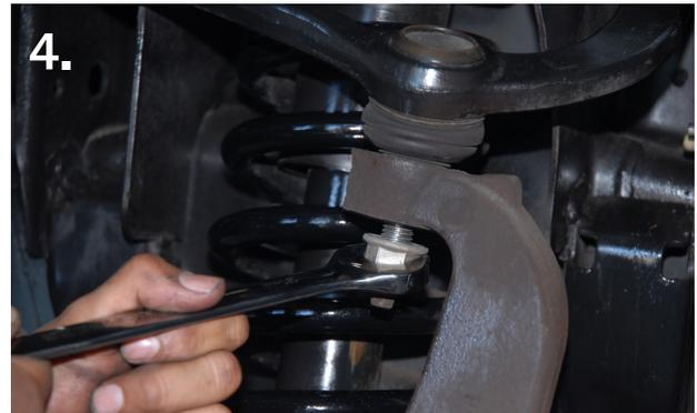
With the top mount nuts removed. Remove upper ball joint nut using a 22 mm socket and or wrench. This will allow for movement of the ball joint to create enough room to remove the stock coil over.
