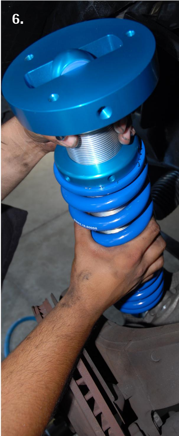
6. Once stock coil over is removed you can then reinstall the new KING coil over shock by tilting the lower end of the shock and with pressure push down until lower shock mount holes are aligned. Then align top mount bolts and hand tighten nuts
