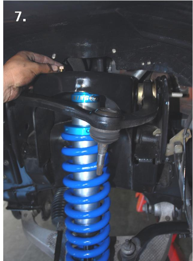
7. Once the shock is in place reinstall ball joint mount and tighten all nuts.
