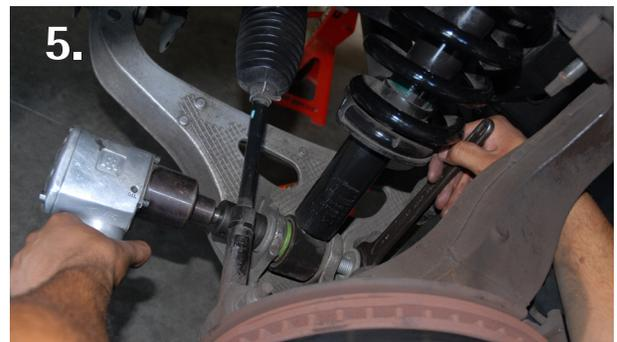
Remove the lower shock mount bolt /nut using a 27mm socket and a 30mm end wrench. With all hardware removed pull down on the stock coil over and remove from A-arm assembly. NOTE: This can be difficult for one person because of the close proximity of the ball joint arm. You may need a second person to help hold the ball joint assembly to one side as you remove the stock coil over.
