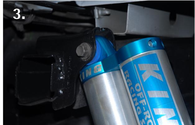
3. Reinstall the new KING shock by aligning the top shock mount and installing the bolt and nut. Do the same process on the lower shock mount. Once the top and lower shock mount bolts have been installed then tighten completely.
