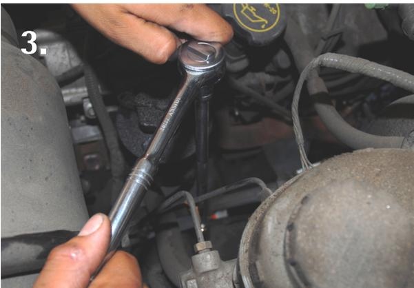
To access the top mounting nuts of the upper shock mount you must open the hood of the vehicle and remove nuts through the engine compartment. Use a 15mm socket with an extension for easy removal.
