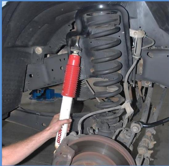
4. To install your new King Shocks remove the nut, washer and upper rubber bushing from the top pin, then Stick the top pin up into the shock mount. Install upper bushing, retaining washer, washer and nut. Thread the nut onto the pin a couple of threads.
