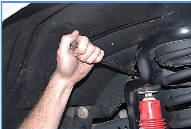
2. Loosen the nut on the lower mount and remove the mounting bolt. Let the shock hang there.
