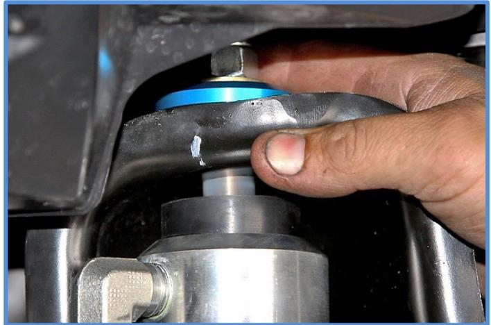
5. Line up the lower shock eye with the mounting holes and slide the lower bolt through. Thread the lower nut onto the bolt.
