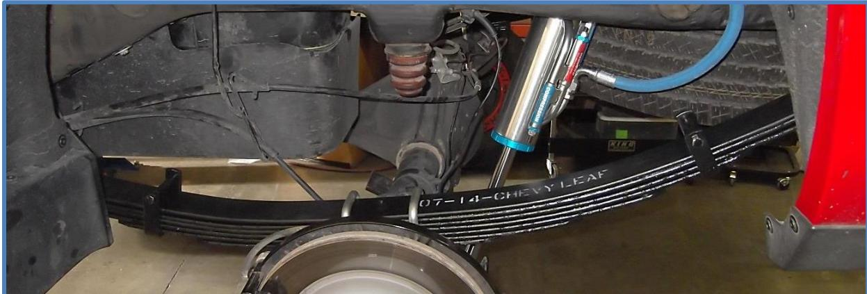
This leaf spring is designed to lift the rear 1"- 1½" over stock without the factory lift block (if applicable). Install leaf springs without the block. Factory lift block can be added if a taller ride height is desired.
