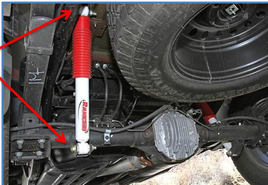
**NOTE:** When installing the new shocks, make sure that you have a driver and passenger side shock. This will insure that the off-set spacers are located in the right direction in order to space the shock away from the frame. Driver-side reservoir should face towards the rear and the passenger-side reservoir should face the front.
