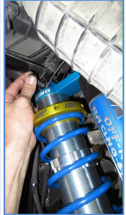
5. Install the factory bolt in the lower mount. Now tighten upper and lower mounting bolts to factory specs.
