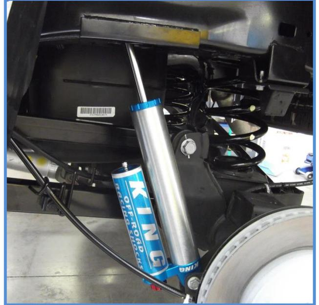
4. On the passenger side (Right side) you may need to pull some slack from the parking brake cable in order to fit the shock. Grab the metal sleeve with pliers and twist the sleeve while pulling the cable through the sleeve. You should only need  $\frac{1}{2}$ " –  $\frac{3}{4}$ " or so, check the fit and adjust accordingly.
