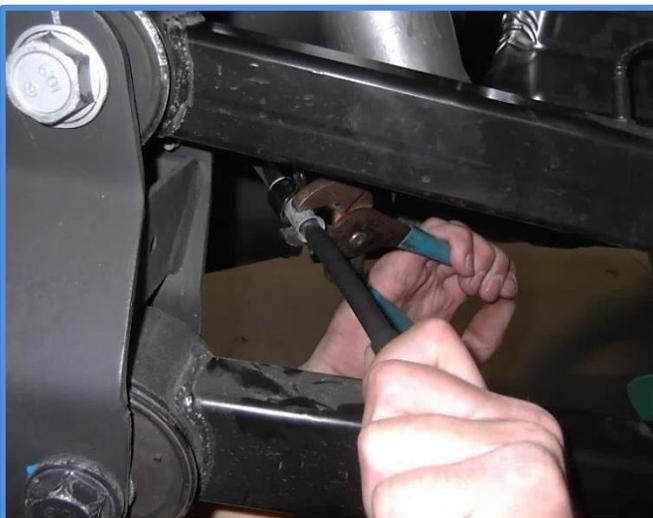
**Important Note:** The rubber bushings on your King shocks are different from each other. Make sure the taller bushing is on the bottom next to the body of the shock as shown. The silver washer between the rubber bushings represents the material thickness of the upper shock mount. It's important to tighten the nut only until the rubber bushings start to compress. There should be approximately  $\frac{1}{8}$ " –  $\frac{3}{16}$ " of the mounting pin protruding above the nut.
