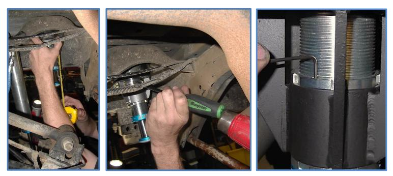
8. Install springs - Unbolt the lower shock mounts, lower the axle enough to install coil springs. Place springs over the bump stop bracket and align with the lower spring perch on axle. Jack axle back up so you can reinstall the lower shock mount hardware. Tighten lower shock mount bolts.
