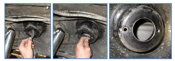
5. Install bump stop brackets – Line up holes in brackets with the nut plate and install the 3/8 x 1" bolts with washer, be sure to use red lock tight. Tighten bolts to 35 ft/lbs.
