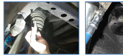
3. Using a 2 <sup>1</sup>/<sub>4</sub>" hole saw, cut a hole in the center of the bump stop mount using the threaded hole in the center as a guide for the pilot bit.
