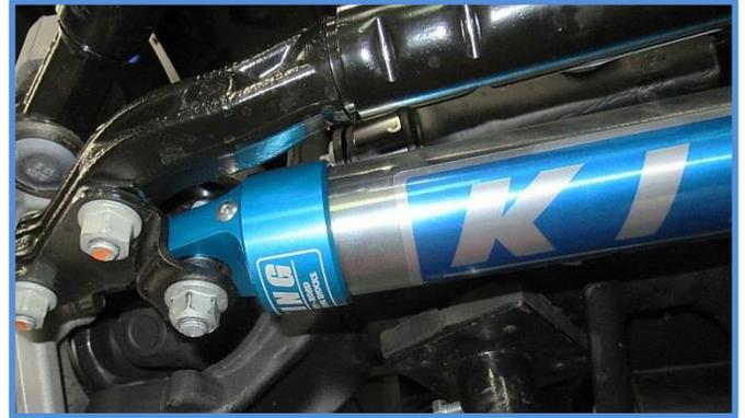
5. Install factory hardware on the axle end and tighten to factory specs.
